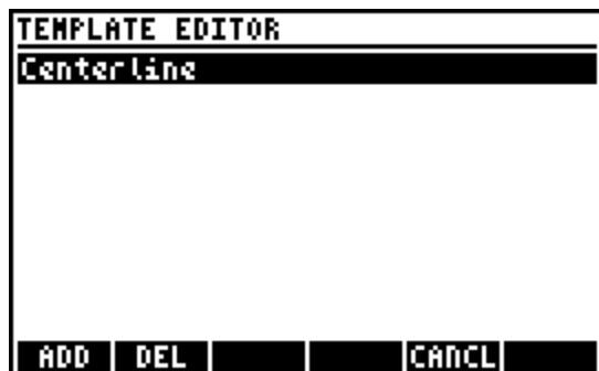
Step 21: Press **ADD** to add an offset, and then enter the width and slope of the offset. All offsets should be entered starting from the centerline and moving away from it. Enter the offsets left, and then right to complete the template.
