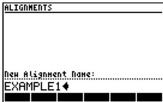
Step 2: Next press **F3 [EDIT]** to edit the newly created alignment. Note: The EDIT HORIZONTAL ALIGNMENT screen always starts by default, use **F6 [HzAL]** to toggle between horizontal/vertical/cross sections.
