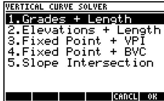
NOTE: BVC = BEGINNING OF VERTICAL CURVE, VPI = VERTICAL POINT OF INTERSECTION, AND EVC = END OF VERTICAL CURVE.
