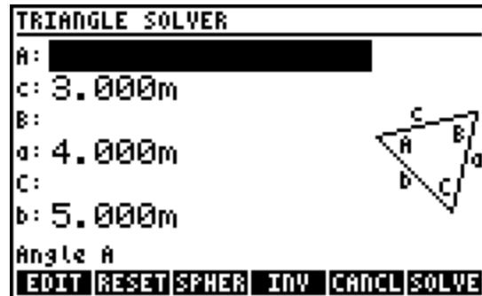
For angle value inputs, the **F4 INV** softkey allows the user to inverse an angle as defined by three points in the job database.
