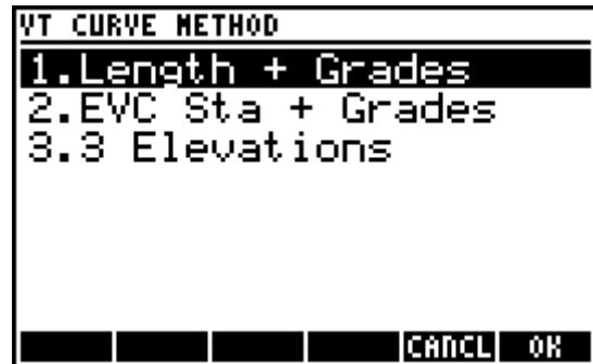
Each of the three methods features a **F4** **SOLVE** softkey to open the horizontal or vertical curve solver to solve for a value. From within the solvers it is possible to export solved values to the clipboard, which can then be pasted into any of the fields in the alignment definition input form.
