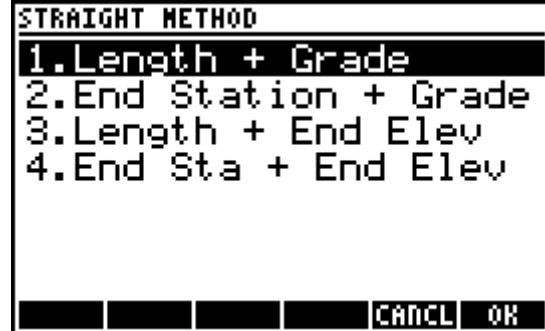
For each of the four methods; the length and end station fields feature a **F4 endHZ** softkey to automatically insert the length or end station to match the end of the horizontal alignment. For methods 3 and 4, the end elevation fields feature a **F4 getZ** softkey to retrieve an elevation from a point in the current job database.
