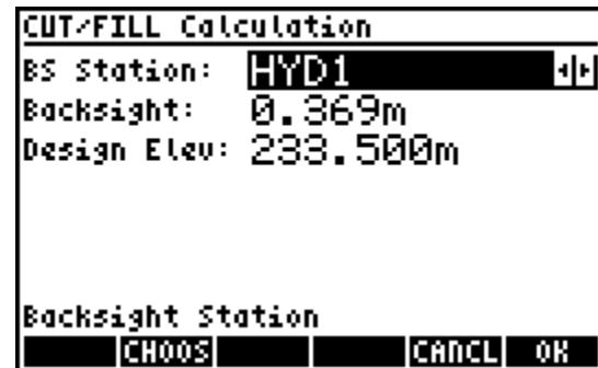
The following input screen displays the target rod reading to meet the design elevation, and prompts the user to input the actual rod reading. The calculation displays the CUT or FILL value and the observed SHOT elevation. The DESIGN elevation and HI values are also displayed for reference purposes.
