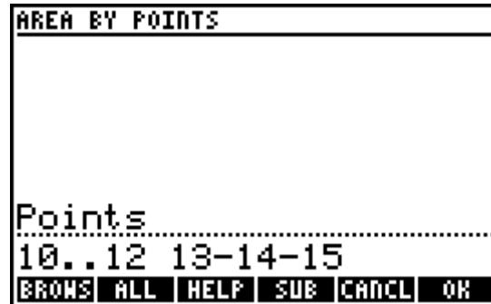
**NOTE: AN ERROR OCCURS WHEN THE POINTS PROVIDED AS CURVE POINTS DO NOT ACTUALLY DEFINE A CURVE, I.E. THE RADIUS DIFFERS BY MORE THAN THE radius tolerance SETTING.**
