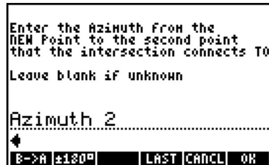
With a known *Distance 1* input there exists a possibility to perform a Distance-Angle intersection. This option is available through the **F3 ANGLE** softkey. The included angle **TO** the second known point at a certain distance from the **FROM POINT** is required for this type of intersection.
