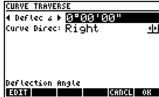
The second field is a Right or Left option for the curve direction. Direction 'Right' is always clockwise, while 'Left' is counter clockwise.
